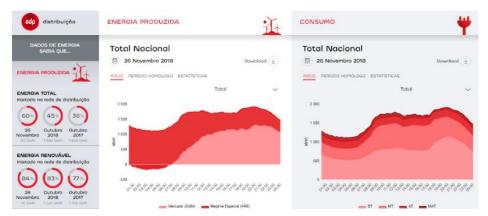
separated by voltage level. The data can be consulted with daily, monthly or yearly aggregation and the stats area of the platform provides an automate comparison with the homologous period. Furthermore, the platform has information regarding the temperature of each day, so that the user can perform a correlation analysis between energy data and temperature.
