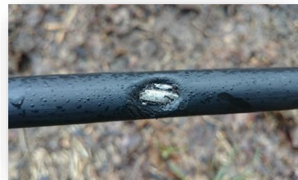
Top pictures: Example of signal (green without fault, red with fault), Bottom pictures: typical fault cause (fallen tree branch) and result (damaged insulation).
