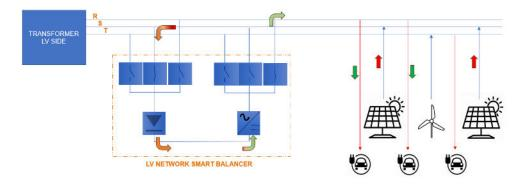
**Working principle**. In this example, the LV Network Smart Balancer allows energy transfer from a high generation phase (S) to a high consumption phase (R).
